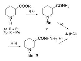
Scheme 2. Reagents and conditions: (i) PhCH<sub>2</sub>Br, Na<sub>2</sub>CO<sub>3</sub>, CH<sub>2</sub>Cl<sub>2</sub>/H<sub>2</sub>O (2/1), reflux, 3 h, 95%; (ii) NH<sub>3</sub> (7N), MeOH, NaCN, 55°C, 2 days, then NH<sub>4</sub>OH (28%), 14 h, 50%; (iii) NH<sub>2</sub>NH<sub>2</sub>·H<sub>2</sub>O (10 equiv.), MeOH, reflux, 4 h, 99%; (iv) NaNO<sub>2</sub>, TFA, H<sub>2</sub>O, 0°C, 1 h, then 80°C, 1 h, 80%. Compound 2 was isolated as its monohydrochloride (precipitated from Et<sub>2</sub>O).
