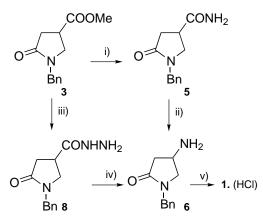
Scheme 1. Reagents and conditions: (i)  $NH_4OH$  (28%), 12 h, 72%; (ii)  $PhI(OAc)_2$ ,  $H_2O/MeCN$  (1/1), rt, 1 h, 75%; (iii)  $NH_2NH_2$ · $H_2O$  (10 equiv.), MeOH, reflux, 2 h, 99%; (iv)  $NaNO_2$ , TFA,  $H_2O$ , 0°C, 1 h, then 80°C, 1 h, 70%; (v) LiAlH<sub>4</sub>, THF, reflux, 3 h, 80%. Compound 1 was isolated as its monohydrochloride (recrystallized from *i*PrOH/*i*Pr<sub>2</sub>O).
